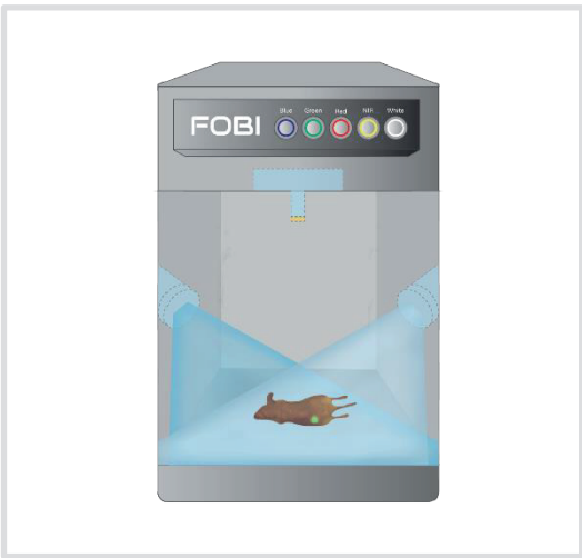
Fig. 2. Structure of FOBI
