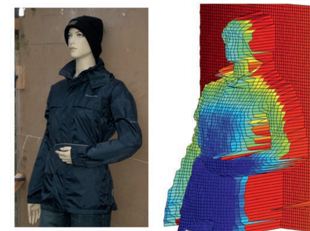
Depth imaging using the single-photon time-of-flight approach with picosecond resolution. The figure illustrates a close-up photograph of a mannequin and a representation of the corresponding cm-resolution depth image when measured at a distance of 325 m under daylight conditions. Data courtesy of G. Buller, Heriot-Watt University, Edinburgh, UK (Opt.Exp. 21, 8907 (2013))
