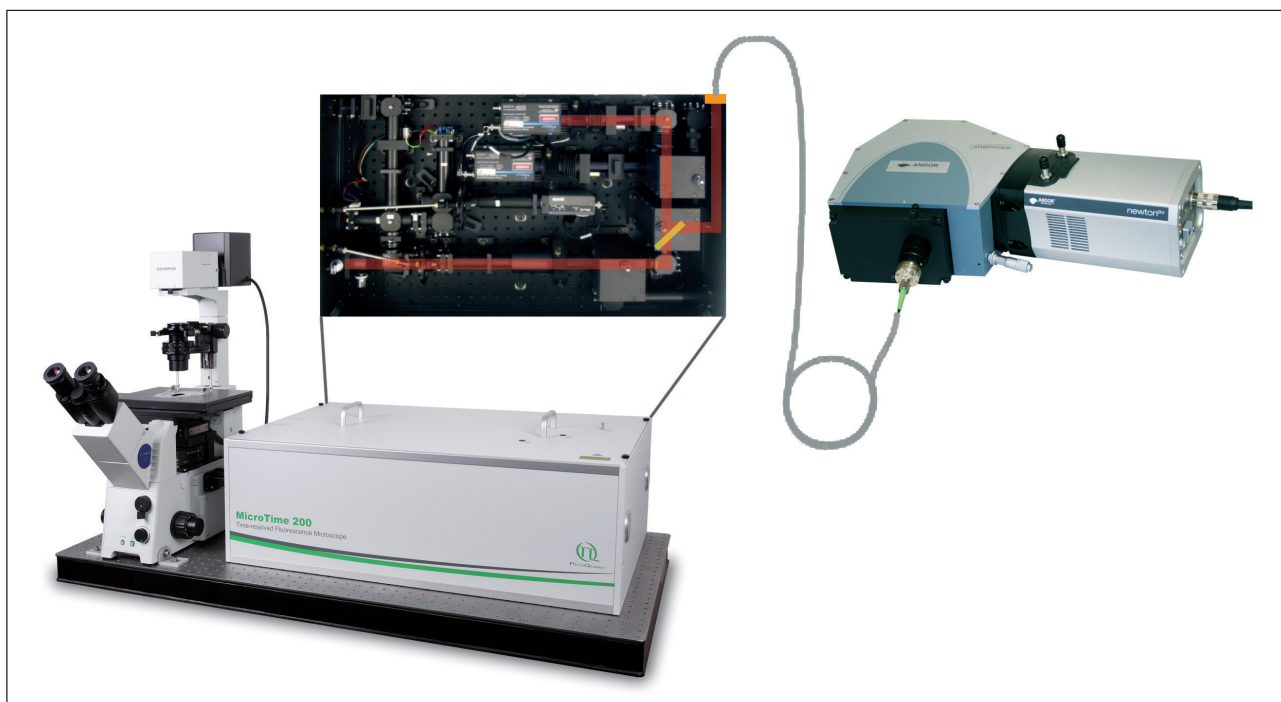
Fig. 1: Graphical presentation of the MicroTime 200 combined with a spectrograph. One example for the fluorescence beampath inside the main optical unit of the MicroTime 200 is shown in red. A beamsplitter (displayed in yellow) defines the part of the fluorescence that is directed towards the exit port (displayed in orange). The fluorescence is coupled into a multimode fiber and directed into the spectrograph SR-163 equipped with a Newton 970 EMCCD (Andor Technology).
