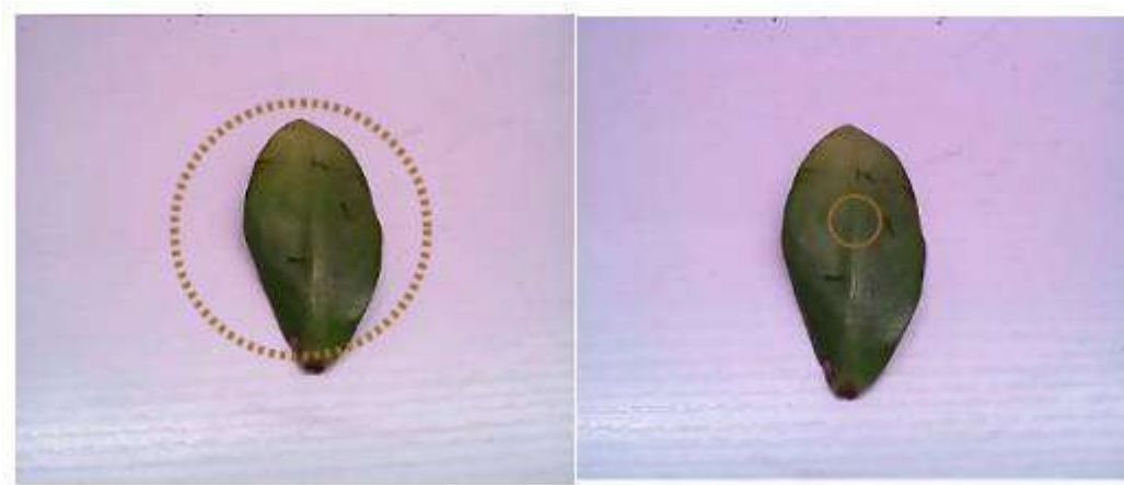
Figure 11 Comparison of Measurement Ranges Between 25° FOV Lens and 5° FOV Lens
