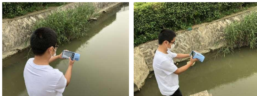
Figure 14 In April 2020, the Aositiancheng ATP9100 ground-based spectrometer monitored the red tide in Sandu Bay, Ningde, Fujian province
