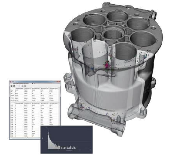
Porosity analysis on compressor housing. Data courtesy of CyXplus
