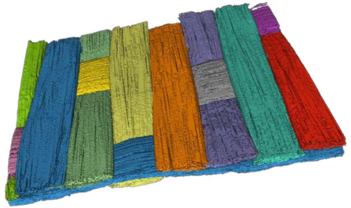
Evolution of damage during fatigue of woven composites.
